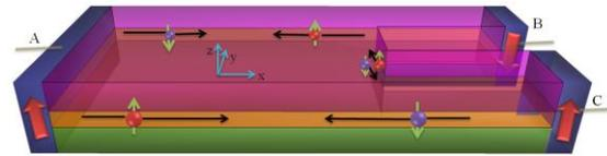
Figure 1: Device Structure. HgTe Quantum Well (middle orange layer) sandwiched between CdTe (green and magenta layers) with thin film magnetic terminals (e.g. CoFeB) (blue) and spin current on edges. Up and Down spin are  $+z$  and  $-z$  polarized respectively.
