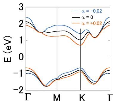
Fig. 2 Lowest conduction band and highest valence band of strained monolayer MoS<sub>2</sub> with  $\alpha = -0.02, 0, +0.02$ .
