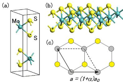
Fig. 1 (a) Bulk unit cell of MoS<sub>2</sub>. (b) Monolayer of MoS<sub>2</sub>. (c) Unit cell of strained monolayer MoS<sub>2</sub> with lattice constant of  $a$ . Parameter  $\alpha$  defines the strain:  $a_0$  is lattice constant of unstrained monolayer MoS<sub>2</sub>, 0.316 nm.
