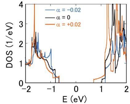
Fig. 3 DOS in unit cell of strained monolayer MoS<sub>2</sub> with  $\alpha = -0.02, 0, +0.02$ .
