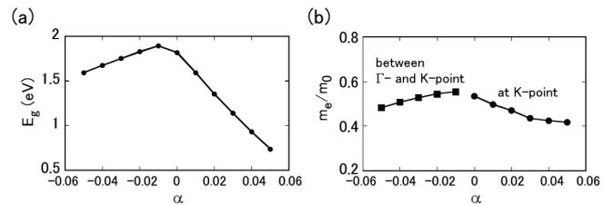
Fig. 4 (a) Dependence of bandgap of strained monolayer MoS<sub>2</sub> on  $\alpha$ . (b) Electron effective mass of strained monolayer MoS<sub>2</sub>. Circular symbols indicate conduction band minimum is at K-point; square ones indicate that it is between K- and  $\Gamma$ -point.
