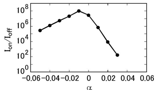
Fig. 6 On-current to off-current ratio for n-channel monolayer MoS<sub>2</sub> FET as a function of strain  $\alpha$ .
