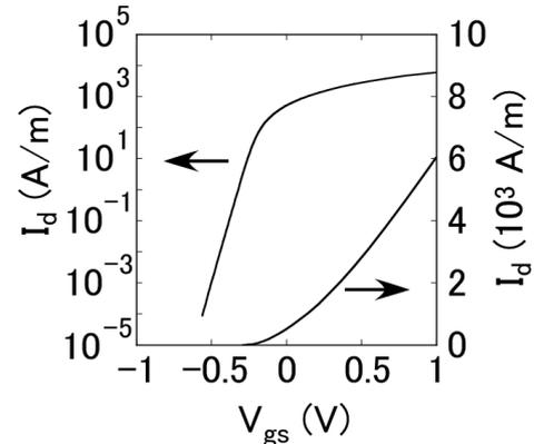
Fig. 5 Calculated transfer curve of n-channel monolayer MoS<sub>2</sub> FET for  $\alpha = 0$ . Drain voltage, gate insulator thickness, and specific permittivity were 1 V, 4 nm, and 16, respectively.
