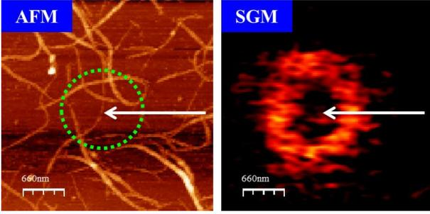
Figure 1 (left) AFM image in a magnified channel region of the SWNT network FET. (right) The corresponding SGM image.
