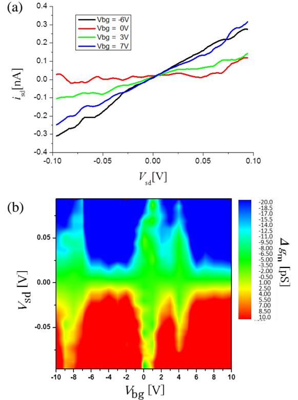
Figure 2 (a) ac component of source-drain current ( $i_{\text{sd}}$ ) versus source-drain voltage ( $V_{\text{sd}}$ ) observed at several fixed back gate voltage of  $V_{\text{bg}} = -6$  V, 0 V, 3 V and 7 V at room temperature. (b) Contour plot of  $i_{\text{sd}}$  as a function of  $V_{\text{bg}}$  and  $V_{\text{sd}}$ . The green color corresponds to a region where the conductance is suppressed.
