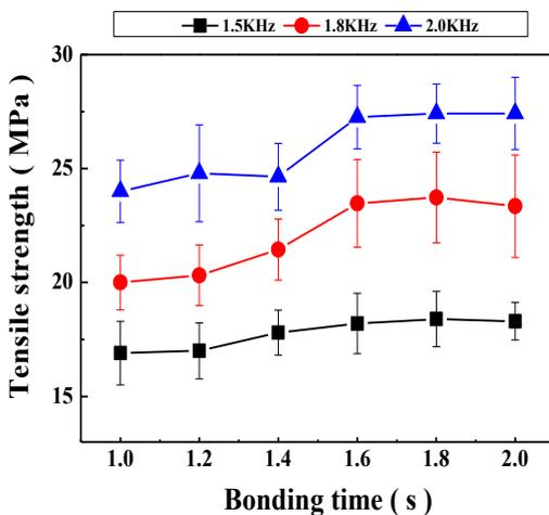
Fig. 2 Tensile strength values of evaluating the pull test in different bonding conditions.
