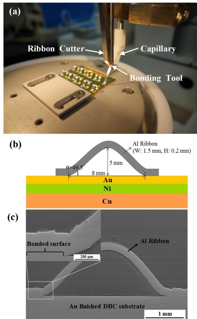
Fig. 1 Schematics of (a) heavy ribbon bonding method; (b) our standard design of ribbon wiring loop, and (c) SEM observation image of a cross-sectioned sample.
