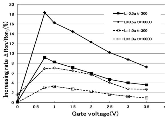
Fig. 4 Dependence of stress gate voltage on the on-resistance degradation rate.
