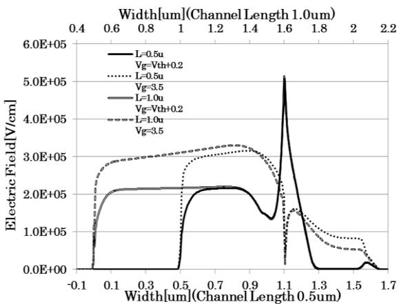
Fig. 1 Comparisons of the Electric field distribution of the thin-film SOI power MOSFETs.
