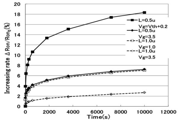
Fig. 5 Dependence of stress time on the on-resistance degradation rate.
