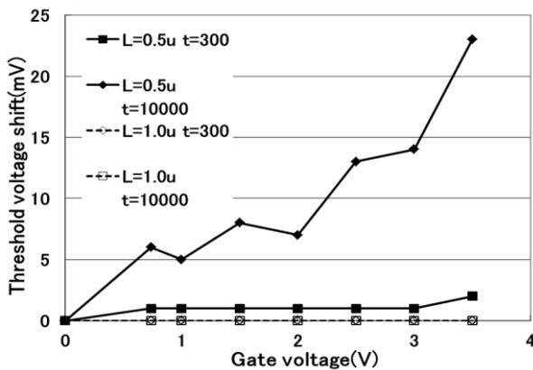
Fig. 3 Dependence of the stress gate voltage on threshold voltage shift.
