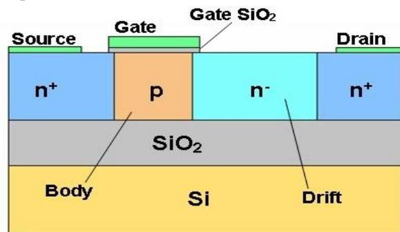
Fig. 2 Schematic cross section of SOI power MOSFET.
