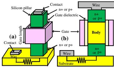
Fig. 1 Structures of vertical MOSFET.
