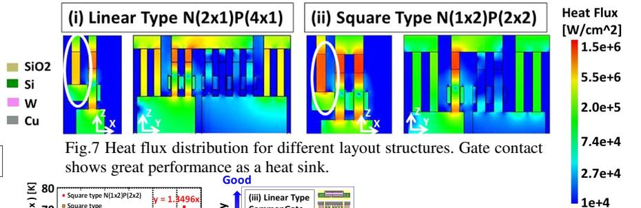
Fig. 7 Heat flux distribution for different layout structures. Gate contact shows great performance as a heat sink.
