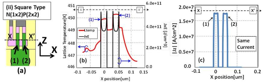
Fig. 6 (a) Square type layout cross-sectional view and (b) the lattice temperature distribution and joule heating, (c) current density for a cross-section line of NMOS drain side.
