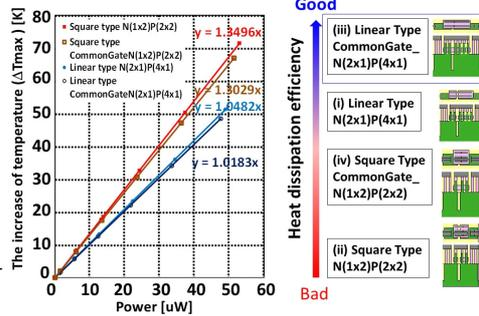
Fig. 8 Thermal resistance ( $R_{th}$ ) of the layout structures. Linear type layout shows higher heat dissipation efficiency compared to the square type layout. Here, the increase of temperature is the difference between the peak temperature and the ambient temperature ( $=400\text{K}$ ).
