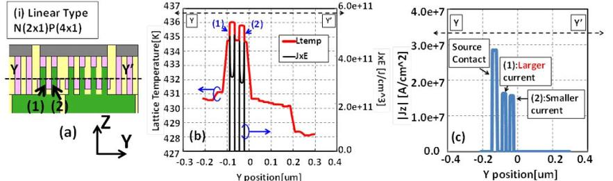
Fig. 5 (a) Linear type layout cross-sectional view and (b) the lattice temperature distribution and joule heating, (c) current density for a cross-section line of NMOS drain side.
