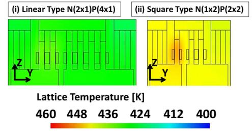
Fig. 4 Lattice temperature distribution for different layout patterns.
