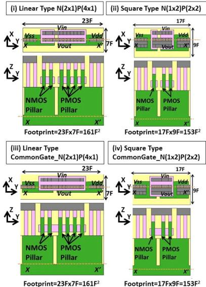
Fig. 2 The simulated layout of CMOS inverter of multi-pillar vertical MOSFET.
