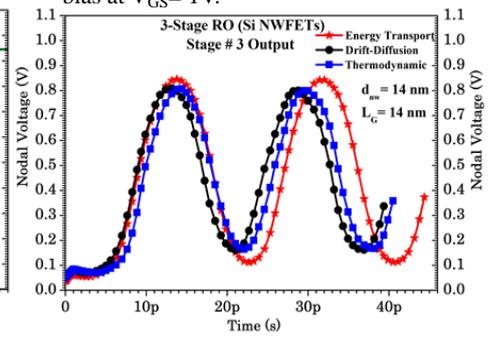
Fig. 10 FO1 3-stage RO nodal output voltage swing for different transport models.
