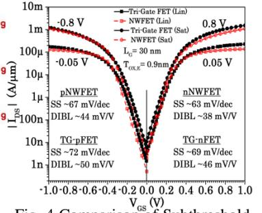
Fig. 4 Comparison of Subthreshold  $I_d$ - $V_{GS}$  of GAA NWFETs with Tri-gate FETs of Intel [6].
