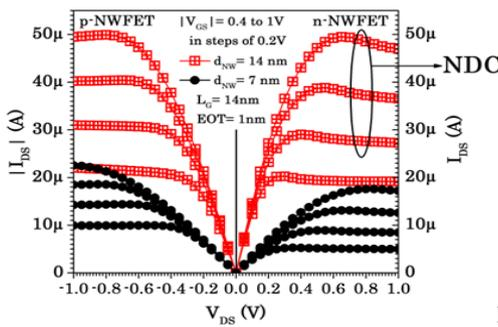
Fig. 6 n-NWFET and p-NWFET output characteristics from energy transport simulations.
