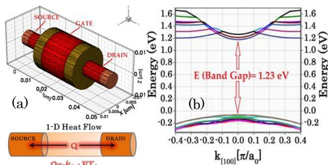
Fig. 1 (a) Si Nanowire FET 3D structure and Schematic of quasi 1-D heat flow in NWFET, (b) Computed electronic energy band structure of 7nm diameter Si nanowire.
