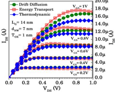
Fig. 5 Output characteristics of 7 nm diameter n-NWFET.
