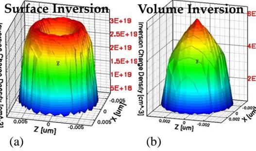
Fig. 3 Quantum corrected inversion charge density in n-NWFET for (a) 14nm and (b) 7nm diameter wires.
