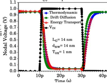
Fig. 9 Si NWFET based inverter pulse response for different transport models.
