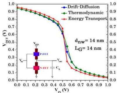
Fig. 8 Si NWFET based CMOS inverter voltage transfer characteristics for different transport models.
