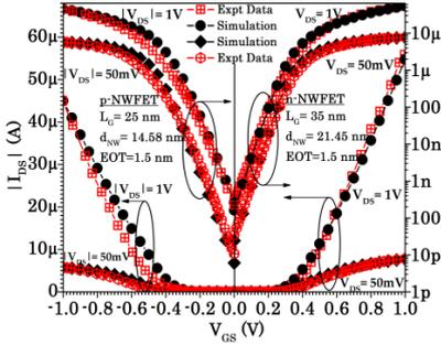
Fig. 2 Calibrated NWFET transfer Characteristics with Expt. Data [5].
