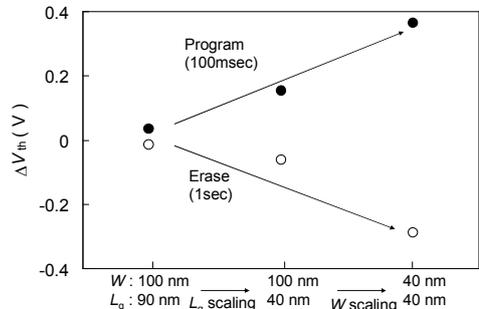
Fig.5  $L_g$  and  $W$  scaling effects on P/E operations. Scaling of  $L_g$  and  $W$  improved both P/E efficiency, which leads to large  $V_{th}$  window
