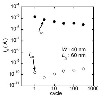
Fig.7 P/E cycle dependence of  $I_{on}/I_{off}$ .  $I_{on}/I_{off}$  ratio of 4 decades was maintained after 300 cycles.
