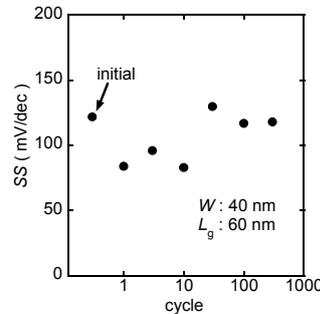
Fig.8 Cycle characteristics of subthreshold slope after each operation.
