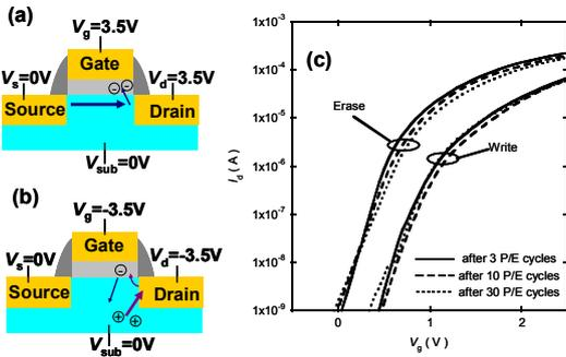
Fig.2  $I_d$ - $V_g$  characteristics of P/E states after 3, 10, and 30 P/E cycles.  $V_{th}$  window of more than 0.3V was repeatedly obtained.
