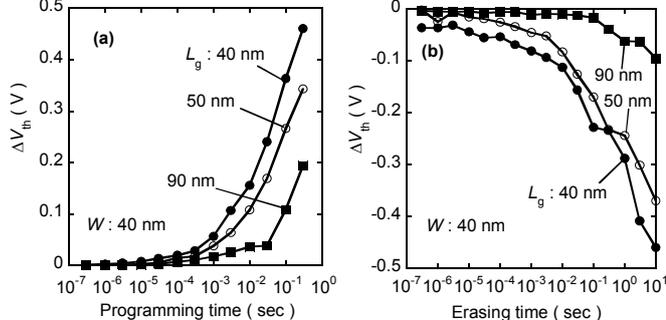
Fig.4 Time dependence of  $\Delta V_{th}$  with different gate length in (a) program and (b) erase operations. Voltage conditions were the same as Fig.3.
