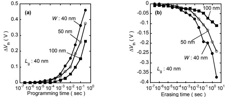
Fig.3 Time dependence of  $\Delta V_{th}$  with different NW width in (a) program and (b) erase operations. Program voltage was set to  $V_g = V_d = 3.5V$ , while erase voltage was set to  $V_g = V_d = -3.5V$ .
