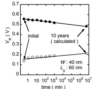
Fig.9 Room temperature data retention after P/E cycles.
