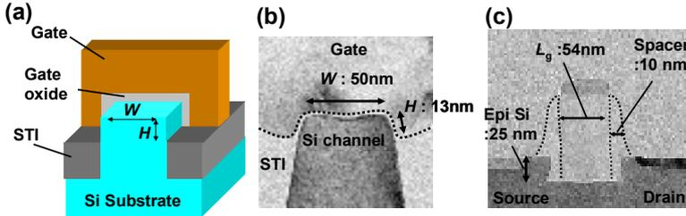
Fig.1 (a) Schematic of Bulk+ Tr. Cross-sectional TEM image along the (b) NW width and (c) gate length direction.
