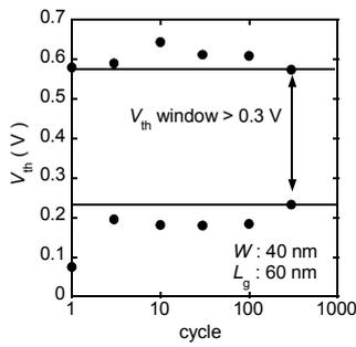
Fig.6 P/E cycle dependence of  $V_{th}$ .  $V_{th}$  window more than 0.3V was obtained after 300 cycles.
