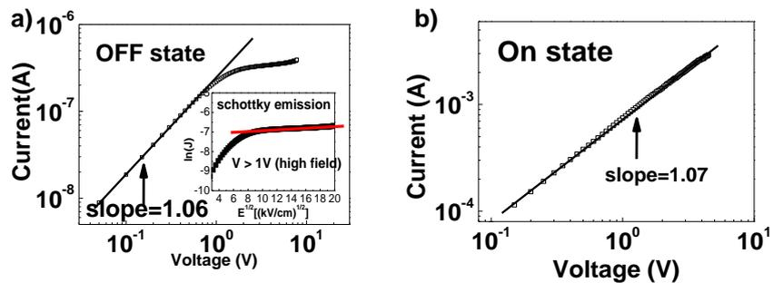
**Fig. 5** a) Experimental and fitted I-V curves of the Al/IGZO/Al WORM devices in the OFF state. The inset shows that schottky emission model is dominant at the high field. b) Experimental and fitted I-V curves of the Al/IGZO/Al WORM devices in the ON state.
