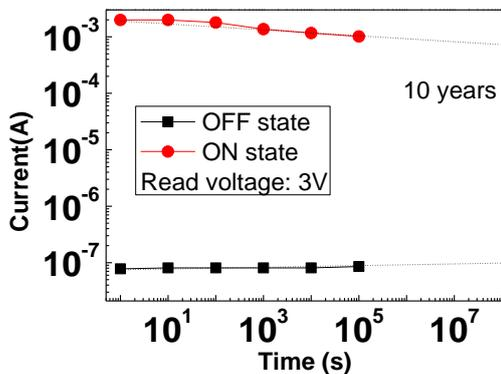
**Fig. 4** Retention characteristic of the OFF- and ON-state of fabricated device read at +3V
