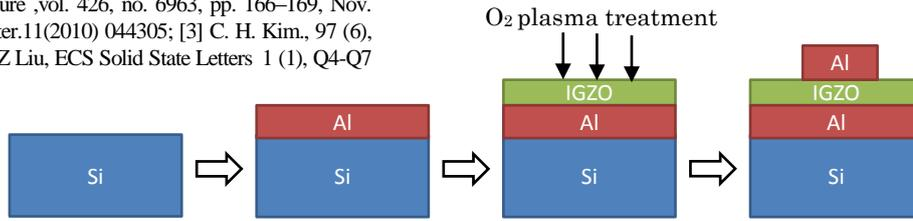
**Fig. 1.** Schematic illustrations of the WORM device process. An 200nm Al and 50nm IGZO film are grown via e-beam and subsequently subjected to O<sub>2</sub> plasma anneal, followed by 200nm Al top electrode via e-beam.
