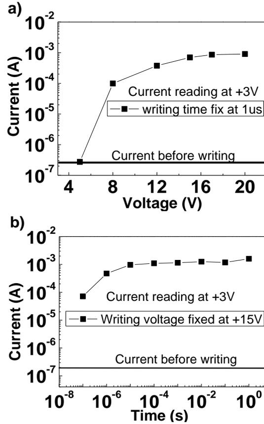
**Fig. 3** Current measured at +3 V as a function of either a) the writing voltage for the fixed writing time of 1  $\mu$ s or b) the writing time for the fixed writing voltage of +15 V.
