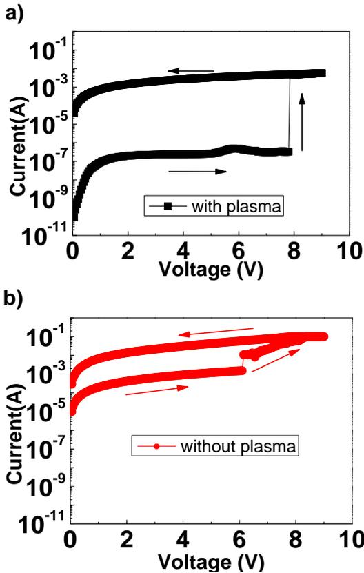
**Fig. 2** Typical I-V characteristics of Al/IGZO/Al devices with and without O<sub>2</sub> plasma immersion by sweeping the voltage from 0 V to 9 V and then back to 0 V on a semi-logarithmic scale.
