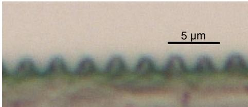
Fig. 3. Cross-sectional image of the fabricated silicone grating.
