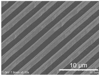
Fig. 2. SEM images of the SiC mold.
