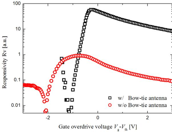
Fig. 3 Experimental results of the Si FET response signal to 0.2 THz radiation. The responsivity has been normalized by maximum value w/o antenna (red circle) with arbitrary unit in order to confirm the relative responsivity results for the effect of antenna.
