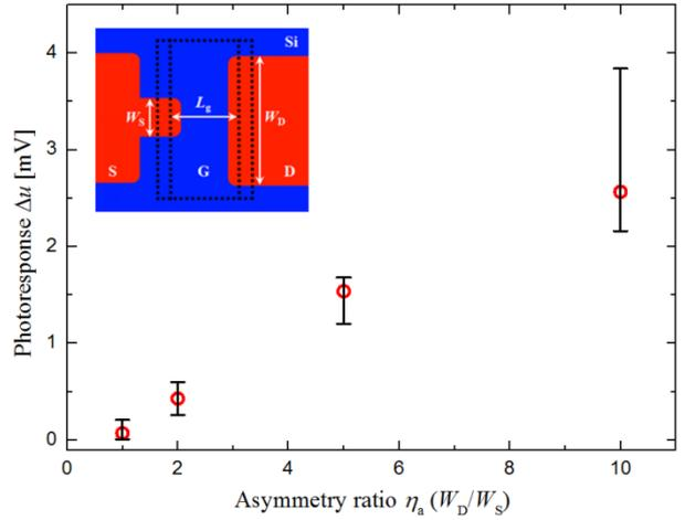
Fig. 5 Experimental results of the photoresponse  $\Delta u$  (mV) for the different asymmetry ratio (Error bars show the sample ranges with standard deviation). Drain width  $W_D = 20 \mu\text{m}$  and source width  $W_S = 2, 4, 10,$  and  $20 \mu\text{m}$  with corresponding asymmetry ratio  $\eta_a = W_D/W_S$  is 10, 5, 2 and 1 (symmetric), respectively.
