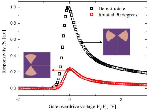
Fig. 4 Responsivity  $R_V$  as a function of  $V_g - V_{th}$  for the polarized THz radiation effects with bow-tie antenna.
