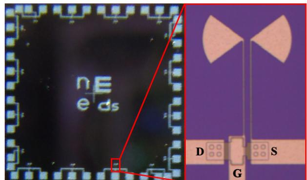
Fig. 2 Photo image of the detector sample. Inset shows Micrograph (top view) of the fabricated Si FET with asymmetric source and drain. The bow-tie antenna has been integrated on electrode metal of gate and source.
