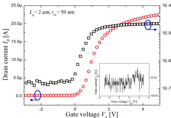
Fig. 1  $I_d$ - $V_g$  curves of the fabricated Si-FETs. The threshold voltage  $V_{th}$  extracted from these DC curves at  $V_d = 1$  V. Inset shows the negligible gate current for all gate voltages.
