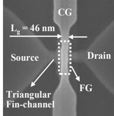
Fig. 2. SEM image of the fabricated floating-gate (FG) type triangular fin-channel flash memory with an ONA-IPD layer (TF-ONA).
