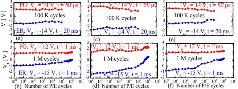
Fig. 11. Endurance characteristics of the fabricated (a)-(b) TF-ONO, (c)-(d) TF-ONA and (e)-(f) RF-ONA devices with the same  $L_g = 46$  nm at different P/E conditions. The TF-ONA device keeps a larger memory window as compared to other devices up to 1 M-cycle operations.
