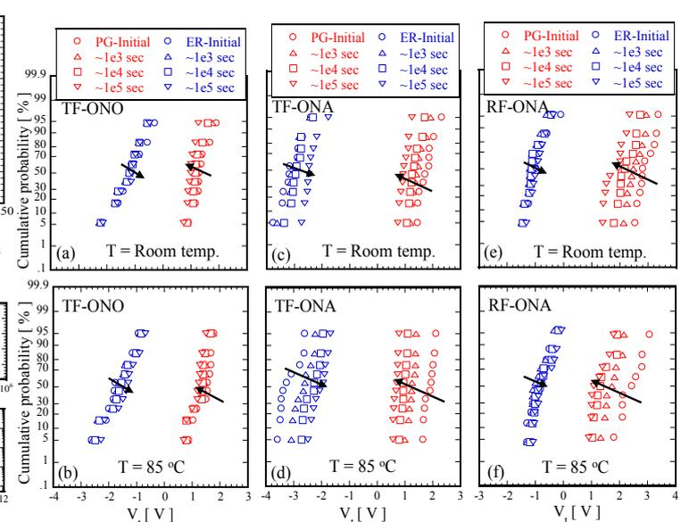
Fig. 12. Data retention of the fabricated (a)-(b) TF-ONO, (c)-(d) TF-ONA, and (e)-(f) RF-ONA devices with the same  $L_g = 46$  nm at room temperature and 85 °C. Data retention for all devices shows a weak dependence on temperature.
