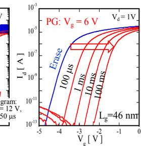
Fig. 7.  $I_d$ - $V_g$  of the TF-ONA device at  $V_g = 6$  V programming with different pulse times.
