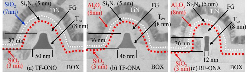
Fig. 3. Cross-sectional STEM images of the fabricated floating-gate (FG) type 3D fin-channel flash memories with different IPD layers and different fin shapes. (a) Triangular-Fin with Oxide-Nitride-Oxide (ONO) IPD layer (TF-ONO), (b) Triangular-Fin with Oxide-Nitride-Al<sub>2</sub>O<sub>3</sub> (ONA) IPD layer (TF-ONA), and (c) Rectangular-Fin with Oxide-Nitride-Al<sub>2</sub>O<sub>3</sub> (ONA) IPD layer (RF-ONA). A 30-nm-thick n<sup>+</sup> poly-Si layer was used as the FG material.
