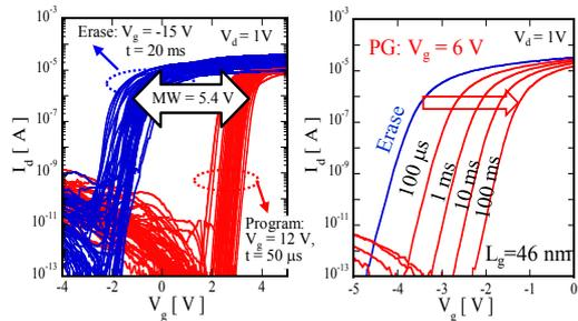
Fig. 6.  $I_d$ - $V_g$  of the fabricated TF-ONA devices with  $L_g = 46$  nm after one P/E cycle.
