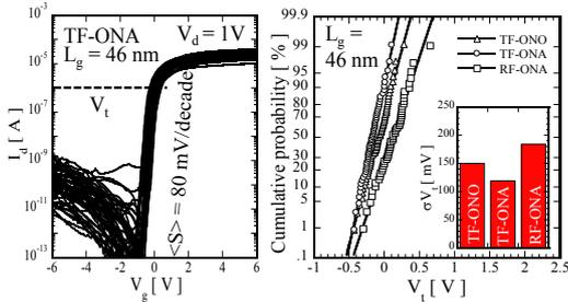
Fig. 4. Initial  $I_d$ - $V_g$  of the fabricated TF-ONA devices with the same  $L_g = 46$  nm.
