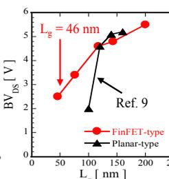
Fig. 9. Comparison of  $BV_{DS}$  and values from FinFET-type and planar-type flash memories.
