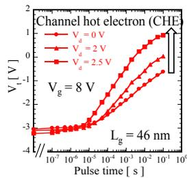
Fig. 8. CHE Programming of the TF-ONA device at different  $V_d$
