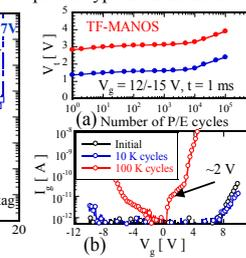
Fig. 14. (a) Endurance and (b)  $I_d$ - $V_g$  of TF-MANOS before and after P/E cycles.
