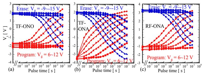
Fig. 10. P/E characteristics of the fabricated (a) TF-ONO, (b) TF-ONA, and (c) RF-ONA devices with the same  $L_g = 46$  nm. It is obvious that TF-ONA device shows a higher P/E speed, a larger memory window and a lower voltage operation due to the high-k and sharp foot edges of a fin.
