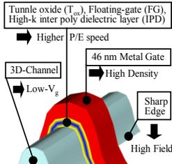
Fig. 1. Device structure of 3D fin-channel floating-gate (FG) type flash memory.
