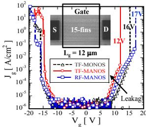
Fig. 13.  $J_g$ - $V_g$  of the fabricated charge trapping type multi-fin devices. Inset is the SEM of the device after fin-EB.
