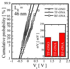
Fig. 5. Statistical  $V_t$  variations of the fabricated 3 kinds of device. Inset is comparison of  $\sigma V_t$  values.
