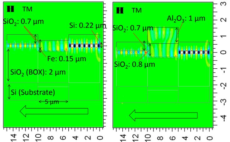
Fig. 5 FDTD simulation on the Fe- $\text{SiO}_2$  DLSPPW with (right) and without (left) the top  $\text{Al}_2\text{O}_3$  layer coupled between SOI waveguides. TM-mode light at the wavelength of  $1.55 \mu\text{m}$  is incident at the right facet.
