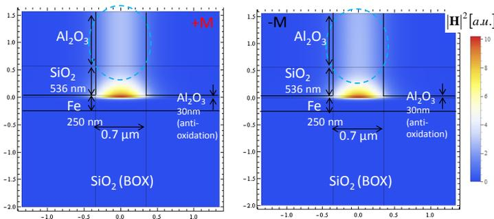
Fig. 4 Optical field profiles of TM mode with magnetization,  $+M$  (left) and  $-M$  (right), in the same structure.
