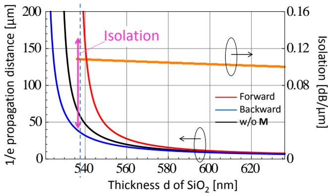
Fig. 3  $1/e$  propagation distance and the isolation as a function of the  $\text{SiO}_2$  film thickness  $d$ . The forward and the backward propagating light are indicated respectively by red and blue curves. The black curve shows the case of no magnetization.
