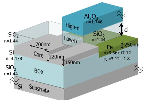
Fig. 2 The front side of the double-dielectric loaded plasmonic isolator coupled with a Si (SOI) waveguide.
