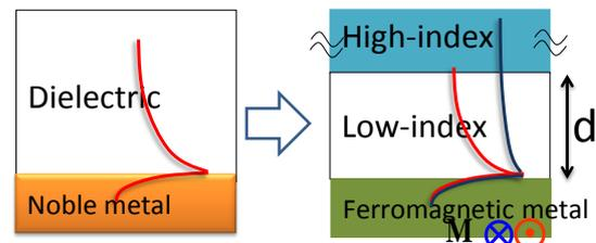
Fig. 1 An application of the SPPs to a plasmonic optical isolator with double-dielectric/ferromagnetic-metal structure.
