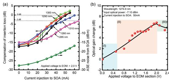
Fig. 3 (a) Insertion loss compensation characteristics of the QD-SOA section in broad wavelength range (1265-1310 nm), and ASE noise from SOA. (b) Typical dependence of optical gain change on DC bias voltage applied to EOM section.
