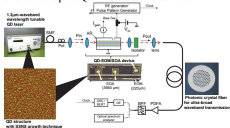
Fig. 2 Opto/electrical setup for characterizing the developed QD-EOM/SOA device, and demonstration of high-speed optical data transmission with the QD-EOM/SOA.
