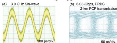
Fig. 4 (a) 3.0-GHz sin-wave form and (b) clear eye opening for 6.0-Gb/s data transmission over 2.0-km-long PCF using QD-EOM/SOA device. Error-free ( $\text{BER} < 10^{-9}$ ) operation was confirmed for 6.0-Gb/s and 2.0-km-long data transmission.
