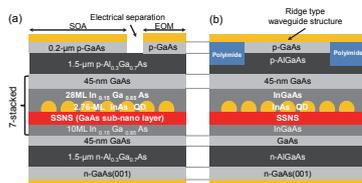
Fig. 1 (a) Side and (b) front schematic images of crystal structure of developed QD-EOM/SOA device.
