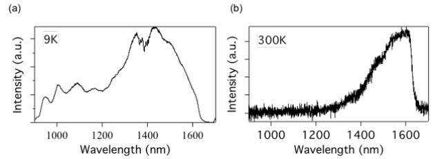
Fig. 3. PL spectra of capped InAs QDs measured at (a) 9 K and (b) 300 K.
