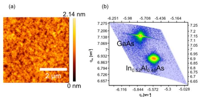
Fig. 1. (a) AFM image of surface of 150-nm  $\text{In}_{0.52}\text{Al}_{0.48}\text{As}$  / InAs / GaAs(111)A, and (b) two dimensional reciprocal space map for 115 reflections GaAs and  $\text{In}_{0.52}\text{Al}_{0.48}\text{As}$ .  $q_{\parallel}$  and  $q_{\perp}$  are the inverse lattice spacing along [111] and [-1-12] directions, respectively.
