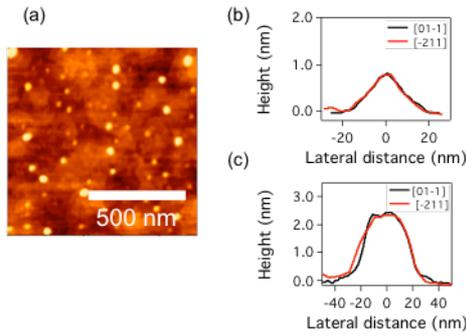
Fig. 2. (a) AFM image of uncapped InAs QDs on  $\text{In}_{0.52}\text{Al}_{0.48}\text{As} / \text{InAs} / \text{GaAs} (111)\text{A}$ , and cross-sectional profile of (b) small QDs and (c) large QDs.
