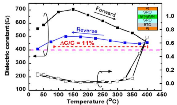
Fig.3 Temperature dependency of dielectric constant and loss (100kHz). The inset shows the sample structure.
