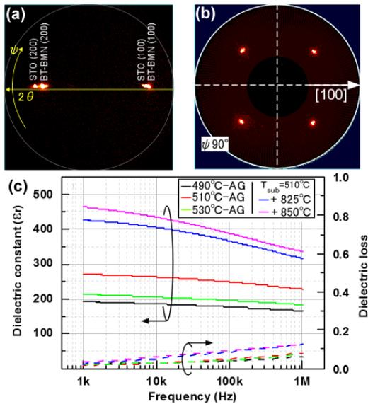
Fig. 1 a) 2D XRD pattern of BT-BMN on STO b) pole figure of {111} reflections on (100) plane and c) dielectric constant as a function of frequency in as-grown (AG) and 825 and 850°C annealed films
