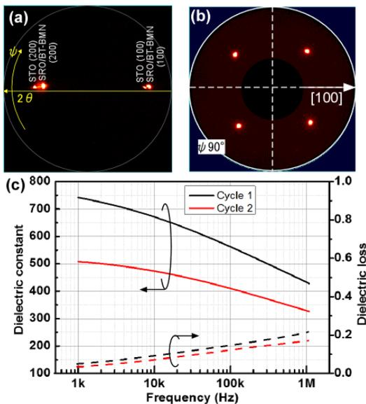
Fig. 2 a) 2D-XRD pattern, b) pole figure projection of {111} reflections on (100) plane and c) frequency dependency of dielectric constant of BT-BMN/SRO/STO structure.
