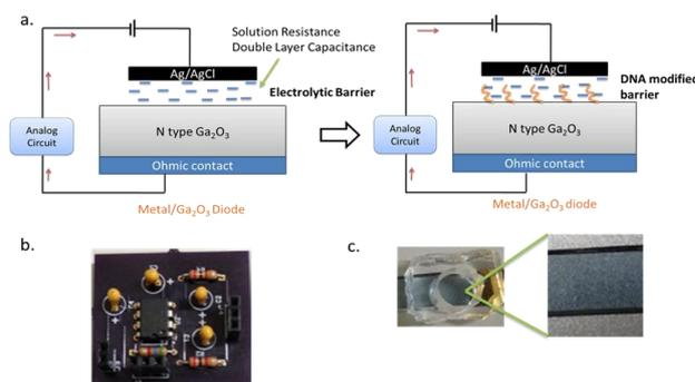
Fig. 3 a. DNA detection through electrolytically interfaced metal/Ga<sub>2</sub>O<sub>3</sub> diode. b. small sensing circuit c. sensing area surrounded by PDMS wall. The inset shows the transparent Ga<sub>2</sub>O<sub>3</sub> sensing surface.
