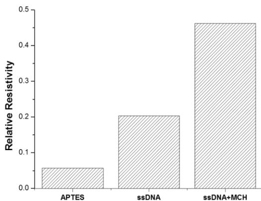
Fig. 5 contribution of each of the surface modifications to the relative resistivity. Each modification increased the resistivity on the functionalized surface.
