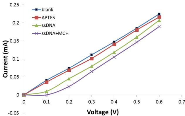
Fig. 4 Surface functionalization with APTES, ssDNA, and MCH observed through shift in current measured after each modification.
