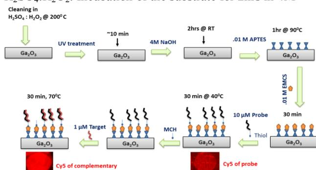
Fig. 1 Functionalization of Ga<sub>2</sub>O<sub>3</sub> surface for DNA sensing. The inset shows the confirmation of functionalization through Cy5 tags.
