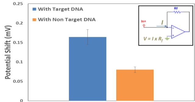
Fig. 7 Average potential shift from immobilization to hybridization for target/non-target DNA. The potential was measured by applying the sensed current to a resistance (inset)
