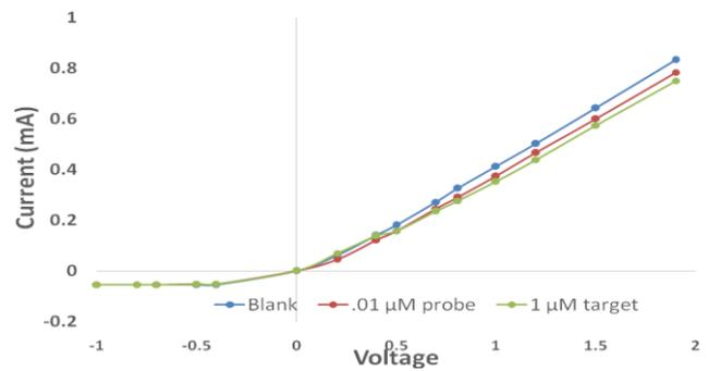
Fig. 6 Current measured on blank Ga<sub>2</sub>O<sub>3</sub> surface, after modification with 0.01 $\mu$ M capture probe DNA and after capture probe DNA was hybridized with 1 $\mu$ M complementary DNA.
