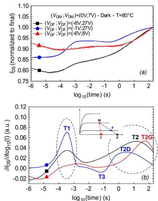
Fig. 1 Drain current transients recorded after trapping in different conditions (see insert).
