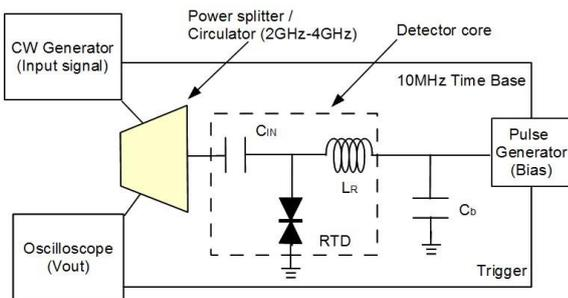
Fig.4 Experimental configuration of the real measurement. .
