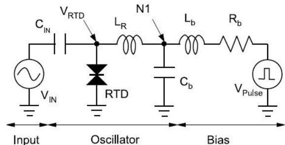
Fig.1 Basic circuit configuration of the super regenerative detector loaded with RTD oscillator.
