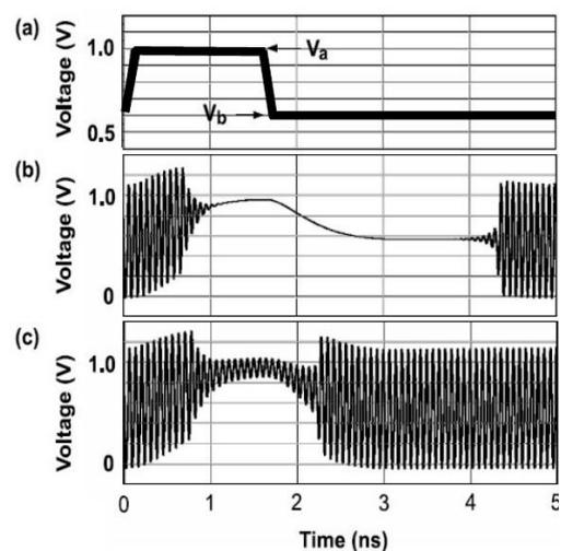
Fig.2 An example of the bias voltage and oscillation waveform of RTD super regenerative detector shown in Fig.1 obtained from circuit simulation.
