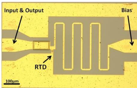
Fig.3 Photograph of the fabricated oscillator load with an RTD.
