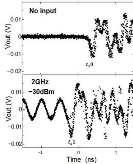
Fig. 5 Output waveforms of the RTD super regenerative detector using circulator for 2GHz signals.
