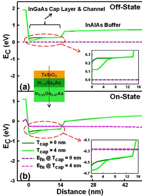
Fig. 3. (a) Off-state and (b) on-state energy band diagrams for the devices with  $x = 0.32$  and different  $T_{cap}$  of 0 and 4 nm. The energy near the channel surface for device with 4-nm-thick capping layer is smaller than that of device without capping layer.
