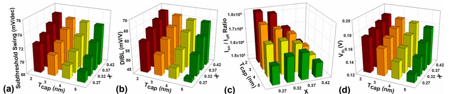
Fig. 7. Plot of (a) subthreshold swing, (b) DIBL, (c)  $I_{on}/I_{off}$  ratio, and (d)  $V_{th}$  versus the  $x$  and  $T_{cap}$ , respectively. Increasing  $T_{cap}$  and decreasing  $x$  of  $In_{(1-x)}Ga_xAs$  will reduce the  $V_{th}$  and improve the subthreshold swing and DIBL; however, there is a trade-off for the variation of  $I_{on}/I_{off}$  ratio.
