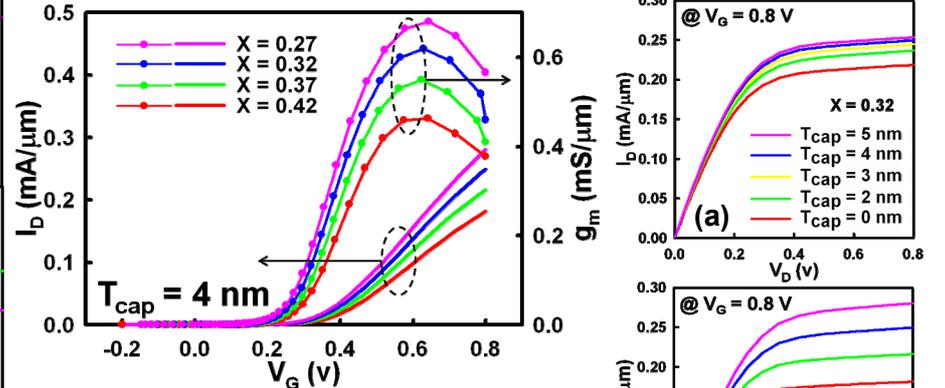
Fig. 4. Plots of  $I_D$ - $V_G$  and  $g_m$ - $V_G$  with different  $x$  and  $T_{cap} = 4$  nm. A small  $x$  implies a low gallium concentration which may reduce the alloy scattering and then increase the channel mobility. Thus, it has higher drive current.
