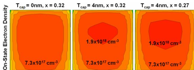
Fig. 6. The on-state electron density.  $T_{cap}$  increases or  $x$  decreases, the electron density increases and the centroid of the inversion charge density in the channel is pulled toward the gate oxide interface.
