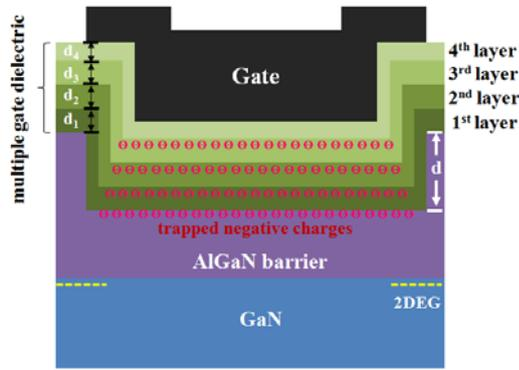
Fig. 1. Schematic of fluorinated multi-gate dielectric structure in the proposed normally-off AlGa<sub>0.25</sub>Ga<sub>0.75</sub>N MIS-HEMTs.
