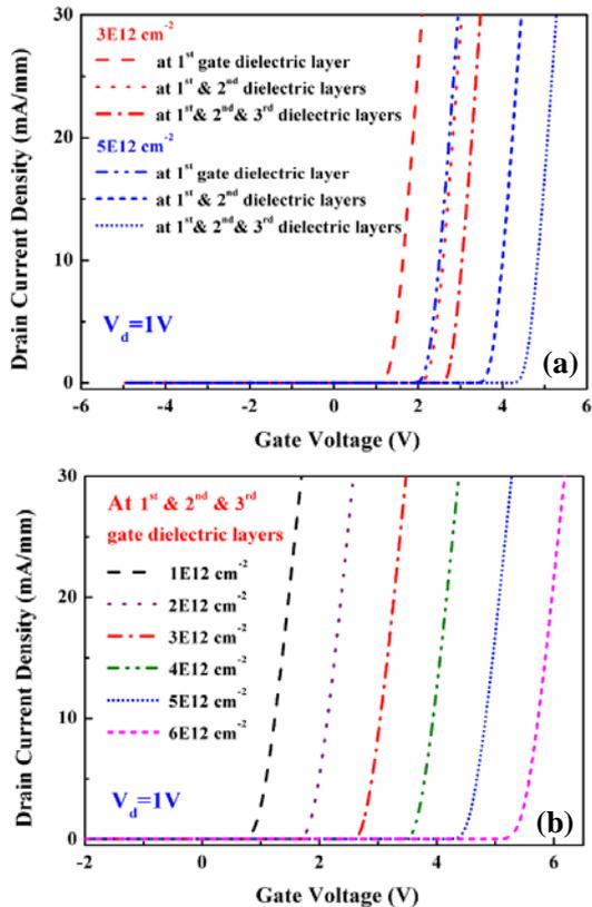
Fig. 2. Dependence of the device transfer characteristics on (a) each dielectric layer at fixed charge density and (b) the fixed negative charge density for each layer in triple fluorinated dielectrics.
