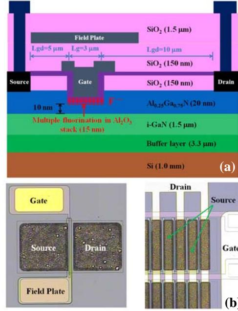
Fig. 3. (a) Device schematic and (b) optical microscopy images of the fabricated normally-off AlGa<sub>0.25</sub>Ga<sub>0.75</sub>N MIS-HEMTs with single gate finger and multiple fingers.
