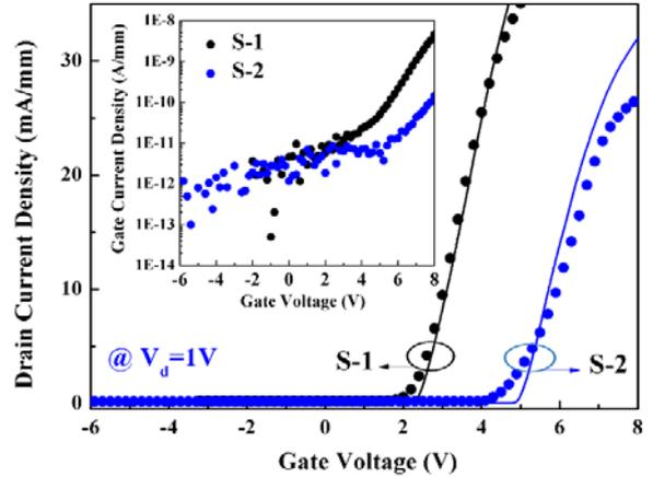
Fig. 4. Transfer characteristics of the simulation (lines) and measurement data (points) on devices S-1 and S-2. The inset shows the gate leakage current of both fabricated devices.
