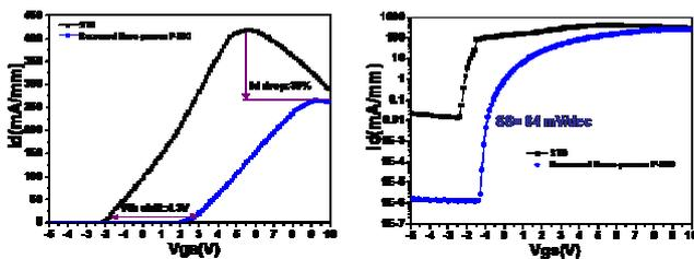
Fig. 3 (a) Comparison of DC transfer characteristics on different GaN-on-Si HEMT devices. (b) show in log scale
