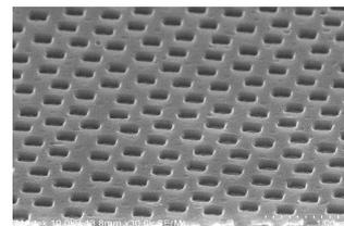
Fig. 2 SEM view of nano-porous structure.
