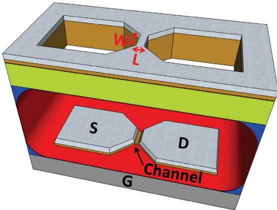
Fig. 2. The perspective view of the fabricated device. The channel length ( $L$ ) and width ( $W$ ) are defined by patterned poly-Si bridge.
