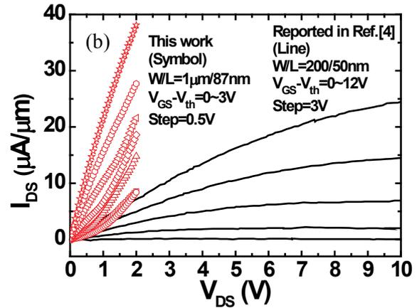
Fig. 4. Comparison of (a) transfer and (b) output characteristics of the FPE IGZO TFT with the 50 nm device reported in Ref. [4].
