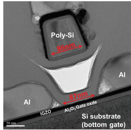
Fig. 3. TEM image of a fabricated FPE IGZO TFT with  $L_{EFF}=87\text{nm}$ .
