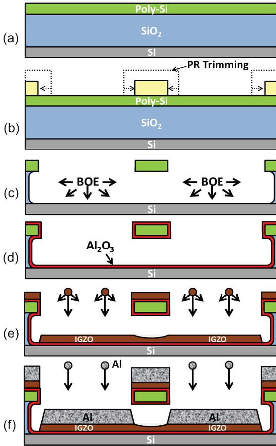
Fig. 1. Process sequence of the fabricated IGZO TFT.
