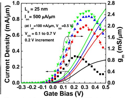
Figure 3: 2.7 nm InAs channel FET:  $I_D$  and  $g_m$ , versus  $V_{GS}$ , at 25 nm  $L_g$ .
