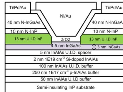
Figure 8: InGaAs MOSFET with recessed undoped InP S/D field spacers
