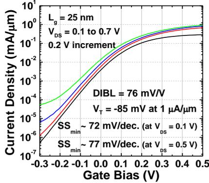
Figure 4: 2.7 nm InAs channel FET: subthreshold characteristics at 25 nm  $L_g$ .
