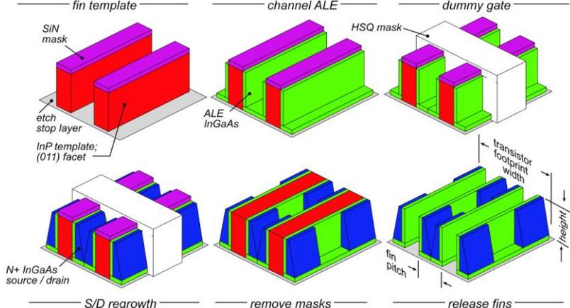
Figure 10: Process flow for high aspect ratio finFETs. The InP template is defined by an wet etch selective to the vertical (011) facet. ALE growth can provide monolayer control of the channel thickness. Not shown: ALD gate dielectric, gate & S/D metals
