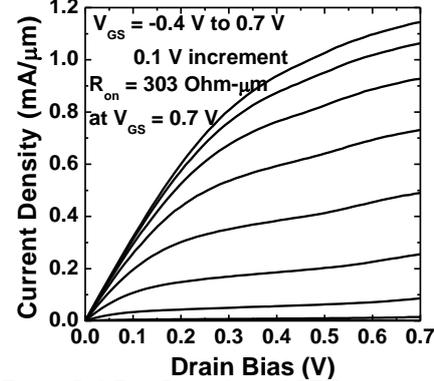
Figure 5: 2.7 nm InAs channel FET: common-source DC characteristics at 25 nm  $L_g$ .
