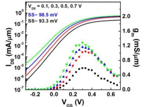
Figure 9: Subthreshold characteristics of the FET of fig. 8. Note the reduced leakage.
