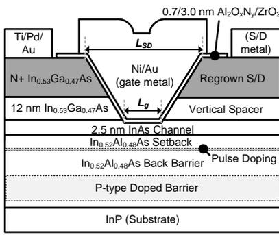
Figure 1: Schematic cross-section of III-V MOSFET with 2.5 nm InAs channel.
