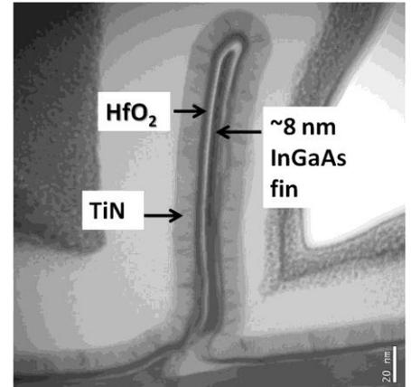
Figure 11: TEM image of a single fin of  $\sim 180$  nm height
