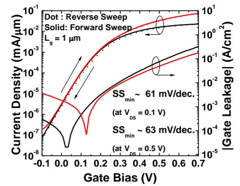
Figure 6: 2.7 nm InAs channel FET:  $\log(I_D)$  and  $\log(I_G)$  versus  $V_{GS}$ , at 1  $\mu\text{m}$   $L_g$ , at  $V_{DS} = 0.1$  V and 0.5 V.
