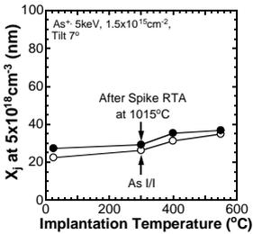
Fig. 6. Junction depth ( $x_j$ ) as a function of implantation temperature. The difference in  $x_j$  before and after annealing becomes smaller with increasing implantation temperature.
