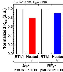
Fig. 11. Normalized  $R_{sd}$  in nMOS and pMOS FinFETs. The normalized  $R_{sd}$  in heated I/I is improved as compared with the RT I/I case.
