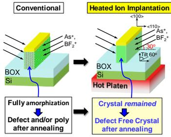
Fig. 1. Schematic illustration of conventional and heated I/I for extension S/D formation in SOI FinFETs. In the case of heated I/I, since the crystallinity is maintained during I/I, the defect-free crystal can be formed by activation annealing.
