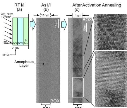
Fig. 3. (a) Schematic illustration of RT I/I in ultrathin SOI layer. (b) and (c) cross sectional TEM images of 11-nm-thick SOI layer after RT I/I and annealing. (a) The I/I conditions were set to the same condition as the ESD formation in FinFETs. (b) The SOI layer is fully amorphized. (c) The polycrystal and twin are observed.
