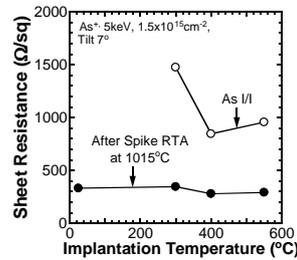
Fig. 7. Sheet resistance as a function of implantation temperature. The sheet resistance of as-implanted can be measured for implantation temperature higher than 300°C.
