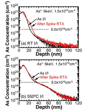
Fig. 5. Arsenic concentration as a function of depth in (a) RT and (b) 550°C I/I.
