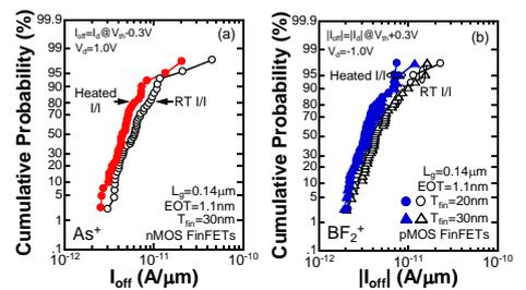
Fig. 12.  $I_{off}$  distribution in (a) nMOS and (b) pMOS FinFETs proceeded by RT I/I or heated I/I with cap layer.  $I_{off}$  in heated I/I becomes lower as compared with that in RT I/I regardless of nMOS and pMOS FinFETs.
