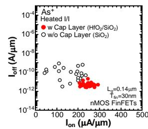
Fig. 9.  $I_{on}$ - $I_{off}$  characteristics in nMOS FinFETs proceeded by heated I/I with and without cap layer. In the case of no cap layer,  $I_{on}$  is lowered and the  $I_{on}$  variation becomes large. In contrast, by capping the fin,  $I_{on}$  gets higher and the  $I_{on}$  variation becomes lower.
