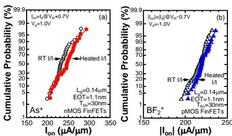
Fig. 10.  $I_{on}$  distribution in (a) nMOS and (b) pMOS FinFETs proceeded by RT I/I or heated I/I with cap layer.  $I_{on}$  in heated I/I is improved as compared with that in RT I/I.
