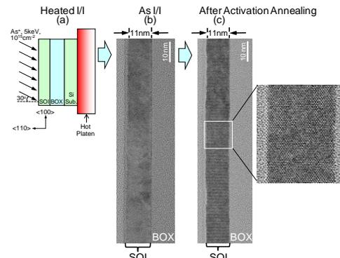
Fig. 4. (a) Schematic illustration of heated I/I in ultrathin SOI layer. (b) and (c) cross sectional TEM images of 11-nm-thick SOI layer after heated I/I and annealing. (b) All SOI layer is maintained the crystal condition. (c) The SOI layer is perfectly crystallized by annealing.
