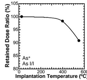
Fig. 8. Retained dose ratio as a function of implantation temperature. From 400°C, the retained dose ratio decreases with increasing implantation temperature, which means that out-diffusion arises during I/I.
