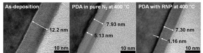
Fig. 2 HRTEM images of as-deposited and annealed  $\text{AlO}_x$  layers.
