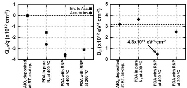
Fig. 1  $Q_{\text{eff}}/q$  and  $D_{it}$  of as-deposited and annealed  $\text{AlO}_x$  layers.
