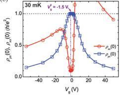
Fig. 1 The QAH effect measured at 30 mK. (a) Magnetic field dependence of  $\rho_{yx}$  at different  $V_g$ s. (b) Dependence of  $\rho_{yx}(0)$  (empty blue squares) and  $\rho_{xx}(0)$  (empty red circles) on  $V_g$ .
