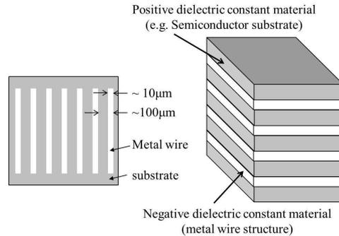
Fig. 3 Schematic of THz region hyperbolic metamaterial
