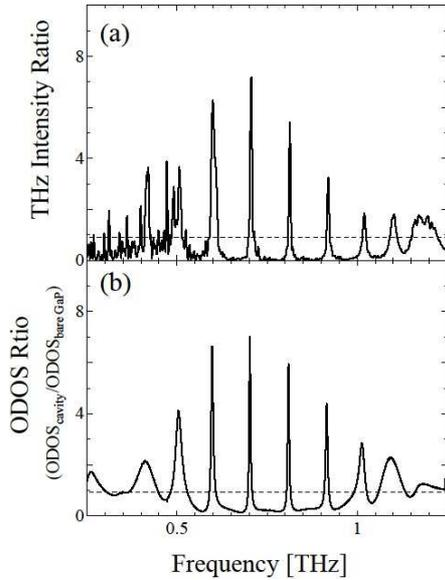
Fig. 2 (a) THz intensity ratio of the experimentally obtained emission spectra, (b) ODOS ratio obtained by transfer matrix calculation. [3]
