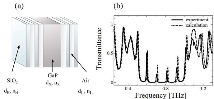
Fig. 1 Schematic of THz region 1D-PC microcavity (a) and its transmission spectrum (b).
