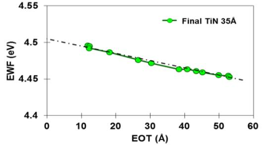
Fig. 3: EWF-EOT curves for SiON bevel with only final TiN
