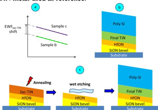
Fig. 1: a) EWF shift induced by sacrificial gates, b) Sample with only Final TiN, c) Sample with also sacrificial TiN metal gates.
