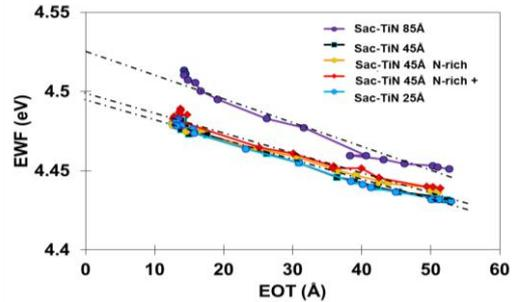
Fig. 4: EWF-EOT curves for SiON bevel with different *sac-TiN* thicknesses and compositions.
