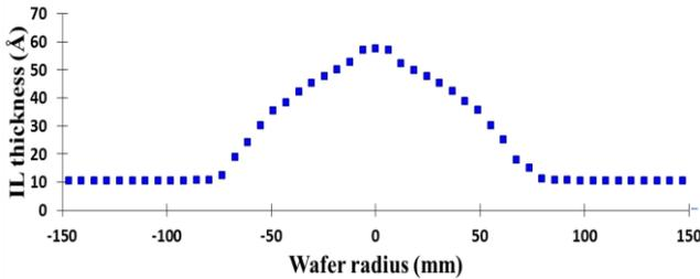
Fig. 2: SiON bevel profile measured by ellipsometry.
