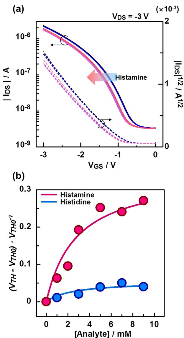
Fig. 2 (a) Transfer characteristics ( $I_{DS}$ - $V_{GS}$ ) of the organic FET upon titration with histamine in a MES-buffer solution (100mM) with NaCl (500 mM) at pH 5.5. [Histamine] = 0-9 mM. (b) Changes in threshold voltage of the organic FET by analytes at various concentrations in a MES-buffer solution (100 mM) with NaCl (500 mM) at pH 5.5. Histamine (●), histidine (●).
