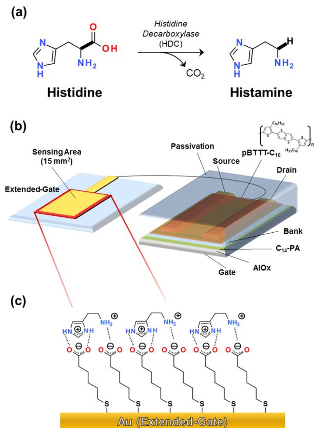
Fig. 1 (a) Biological conversion of histidine to histamine by bacteria with histidine decarboxylase in fish. The amount of histamine is one of the freshness criteria. (b) Schematic structure of the designed extended-gate type organic FET. (c) A plausible model for histamine recognition.
