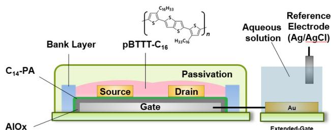
Fig. 1 Schematic structure of the designed extended-gate type organic FET.
