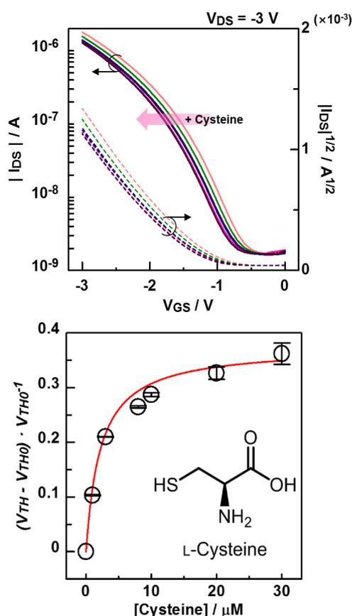
Fig. 2 Top: Transfer characteristics ( $I_{DS}$ - $V_{GS}$ ) of the organic FET upon titration with cysteine in a HEPES buffer solution (10 mM) with NaCl (100 mM) at pH 7.4. [Cysteine] = 0-30  $\mu\text{M}$ . Bottom: Threshold voltage of the organic FET by cysteine at various concentrations in a HEPES buffer solution (10 mM) with NaCl (100 mM) at pH 7.4.
