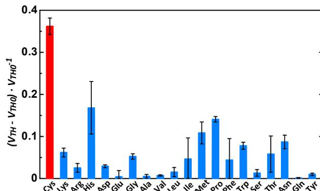
Fig. 3 Threshold voltage changes in the fabricated organic FET-sensor after addition of amino acids in a HEPES buffer solution (10 mM) with NaCl (100 mM) at pH 7.4. [Amino acid] = 30  $\mu\text{M}$ .
