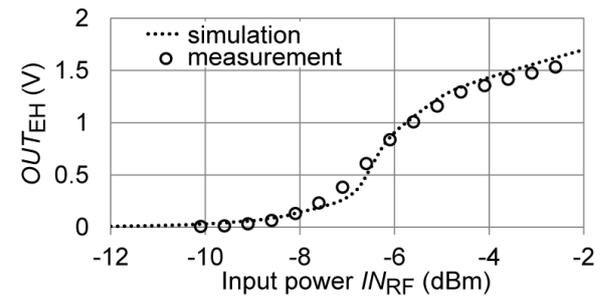
Fig. 5 Measurement and simulation results of  $OUT_{EH}$  versus input power  $IN_{RF}$  at 915MHz
