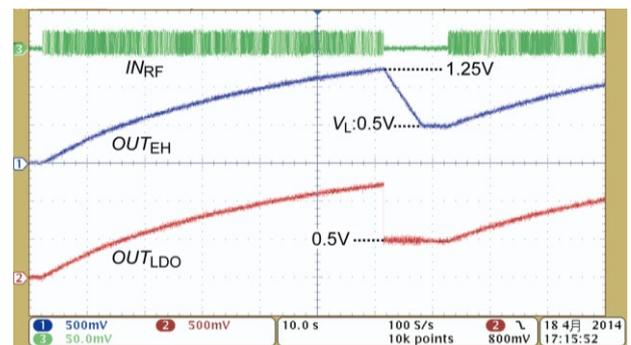
Fig. 7 Measurement results of  $IN_{RF}$ ,  $OUT_{EH}$  and  $OUT_{LDO}$  versus time at -3.6dBm input power
