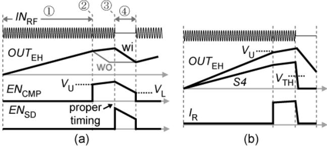
Fig. 2 (a) Timing diagram of the power management circuit
