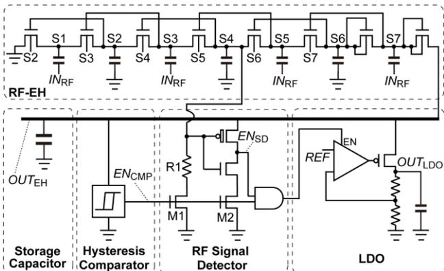
Fig. 3 Schematic of the proposed power management system
