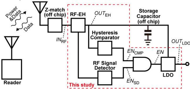
Fig. 1 Block diagram of the proposed power management system
