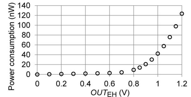
Fig. 6 Measurement results of power consumption versus  $OUT_{EH}$
