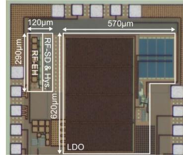
Fig. 4 Chip micrograph of fabricated circuit in Si CMOS 180nm
