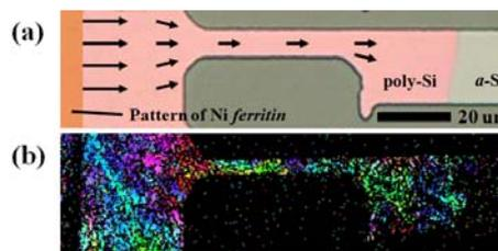
Fig. 2 (a) Micrograph of the resonators after MILC and (b) EBSD image of same area. The Si film is crystallized along the direction of arrows from the pattern of *apoferritin* with Ni NPs.
