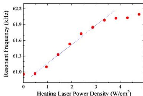
Fig. 5 Resonant frequencies as a function of heating laser power.
