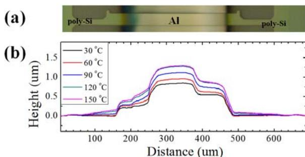
Fig. 3 (a) Micrograph of the resonator surface and (b) its cross-sectional profile as a function of substrate temperature.
