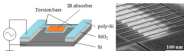
Fig. 1 Schematic diagram of a vibrational MEMS IR sensor (left) and SEM image of the fabricated device (right).
