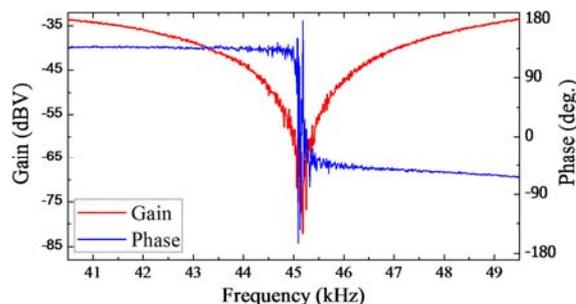
Fig. 4 Resonant curves of the fabricated resonator.
