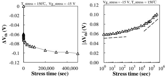
Fig. 1 Time dependence of typical  $\Delta V_{th}$  of a SiC MOSFET under a negative bias.
