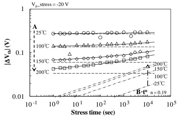
Fig. 5 Time dependences of  $\Delta V_{th}$  of SiC MOSFETs at varied temperatures.
