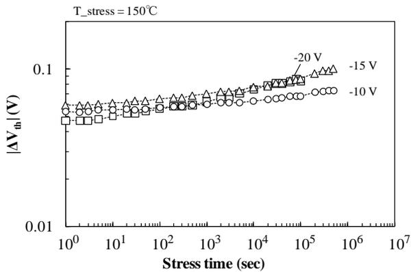
Fig. 4 Time dependence of  $\Delta V_{th}$  of SiC MOSFETs under various negative stress biases at stress temperature of 150°C.
