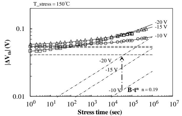
Fig. 6 Time dependence of  $\Delta V_{th}$  of SiC MOSFETs under various negative stress biases at stress temperature of 150°C.
