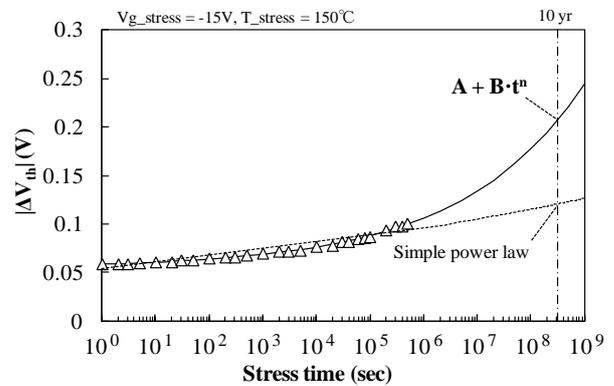
Fig. 8 Long term estimation of  $\Delta V_{th}$  of SiC MOSFET under negative bias using two-component model.
