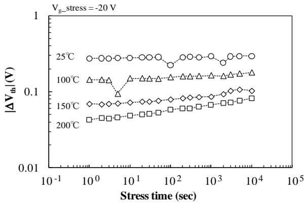
Fig. 3 Time dependences of  $\Delta V_{th}$  of SiC MOSFETs at varied temperatures.
