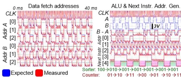
Figure 4. CNT computer output waveform, showing correct operation. This waveform shows the computer performing integer sorting and integer counting concurrently. The CNT computer implements non-pre-emptive multi-tasking, whereby each process voluntarily performs a self-interrupt and gives control to the other task.
