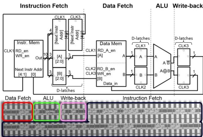
Figure 3. CNT computer. Top: schematic of CNT computer, composed of 4 sub-units: instruction fetch, data fetch, arithmetic unit (ALU), and write-back stage. Bottom: Scanning electron microscopy image of a CNT computer.
