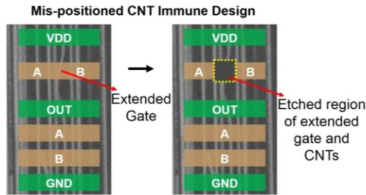
Figure 1. Mis-positioned CNT-immune design for a NAND2. An etch region defined within the standard cell renders the logic gate immune to any mis-positioned CNTs.
