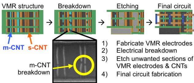
Figure 2. Schematic illustrations of VMR design and process flow. Details of the process can be found in [5].
