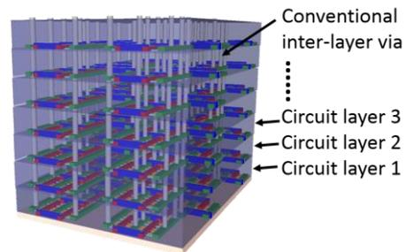
Figure 5. Schematic of a monolithic 3D IC. Multiple layers of circuits are fabricated directly over previous layer of circuits, using the same substrate. The circuit layers are connected with minimum-size vias rather than larger TSVs.
