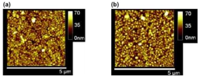
Fig.3 AFM image of DNTT surface (a) without parylene annealing and (b) with parylene annealing.
