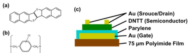
Fig.1 The chemical structures of (a) DNTT and (b) parylene. (c) Structure of bottom-gate top-contact OTFT
