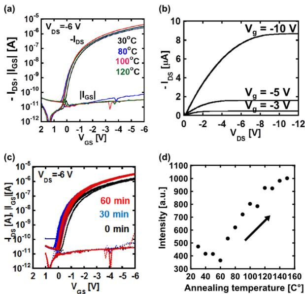
Fig.2(a) Transfer characteristics of device. (b) Output characteristics of device. (c) Device performance change with annealing time. (d) XRD peak intensity dependence at  $2\theta = 14.5^\circ$  with annealing temperature.
