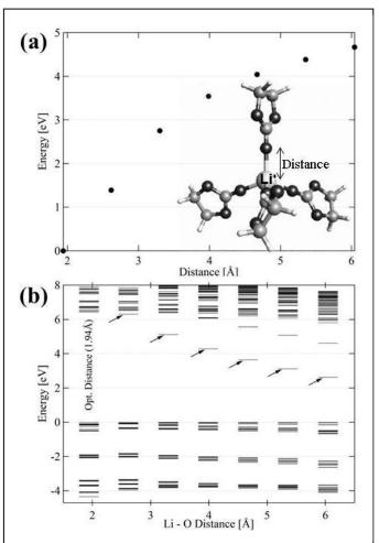
Fig. 1 (a) Total energy variation for a tetrahedral coordination of a lithium ion and four ECs as a function of distance between the lithium and the ECs. (b) The orbital energy variation of the system near the Fermi level as a function of distance between lithium atom and oxygen atoms of ECs.
