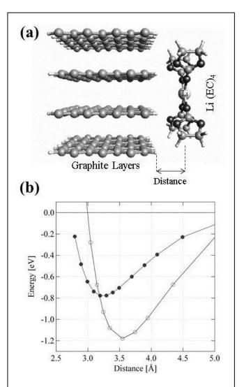
Fig. 2 (a) Schematic view of the graphite edge with hydrogen termination and  $\text{Li}(\text{EC})_4$  molecule in the unitcell of current calculations. (b) Total energy variation as a function of distance between graphite and Li(EC)4 with hydrogen termination (filled circles) and oxygen termination (open circles).
