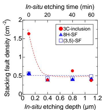
Fig. 1 SF densities for the *in-situ* etching depth or *in-situ* etching time.
