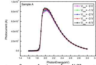
Fig. 4 PC spectra of sample A under different bias voltages
