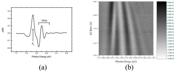
Fig. 1 ER spectra of sample A GaInP solar cell (a) at 0V (b) ERBW mapping
