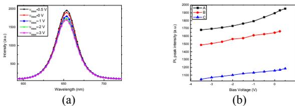
Fig. 3 (a) PL spectra of sample A at different bias voltages (b) PL peak intensity at different bias voltages.
