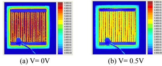
Fig. 5 LBIC mapping of sample A with different bias voltage
