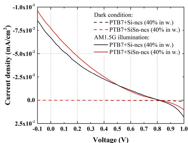
Fig. 2 presents the current-voltage characteristics of hybrid solar cells using 25mg of PTB7 mixed with 40% in weight of SiSn-ncs or Si-ncs as active layer under AM1.5G (solid lines) and dark condition (dashed lines).
