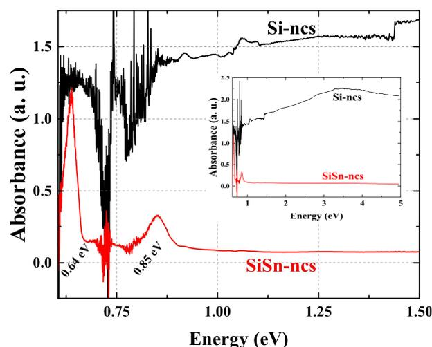
Fig. 1 presents the absorbance spectra of SiSn-ncs (red line) compared to Si-ncs (black line) dispersed in ethanol. The embedded graph corresponds to the same absorbance spectra at wider energy scale from 0.6 until 5eV.
