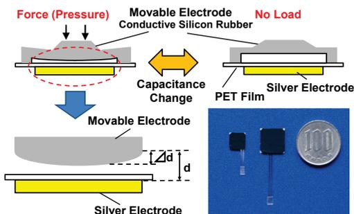
Fig. 1 A schematic cross section and a photograph of a flexible capacitive pressure sensor [2].
