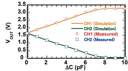
Fig. 9 Capacitance change  $\Delta C$  dependence of  $V_{OUT}$ .
