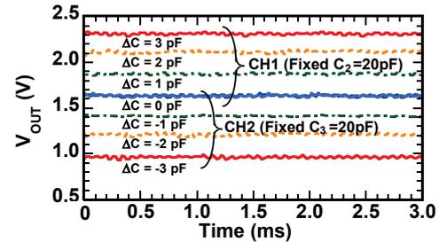
Fig. 8 CV converter output  $V_{OUT}$  for  $\Delta C = \pm 3$  pF.
