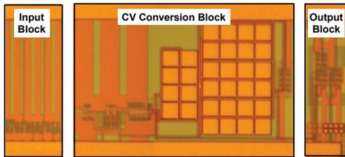
Fig. 6 Photographs of circuit blocks of 2 channel CV converter.
