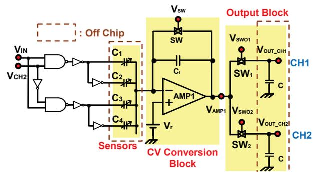
Fig. 3 Proposed 2 channel CV converter circuit.
