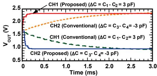
Fig. 5 Simulated waveforms of  $V_{OUT}$  for the conventional and proposed circuits.
