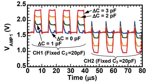
Fig. 7 Measured results of  $V_{AMP1}$  for various  $C_1$  for fixed  $C_2$ .
