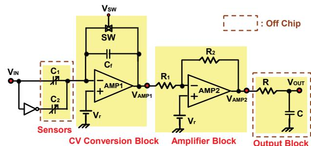
Fig. 2 Conventional single channel CV converter circuit [3].
