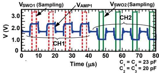
Fig. 4 HSPICE simulation result of  $V_{AMP1}$  and sampling signals  $V_{SWO1}/V_{SWO2}$ , which capture the proper voltage of  $V_{AMP1}$ .
