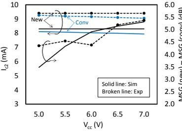
Fig.8 First investigation of bias condition on power gain difference at high  $V_{cc2}$  and low  $I_b$
