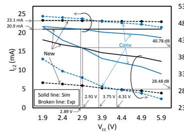
Fig.9 Second investigation of bias condition on power gain at low  $V_{cc2}$  and high  $I_b$
