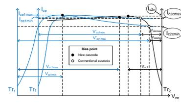
Fig.4 First analysis at high  $V_{cc2}$  on static IV characteristic. New cascode with both two transistors operated in active mode shows higher second-stage collector bias current  $I_{c2}$  than that of conventional one with bias condition of having one transistor in saturation region.
