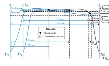
Fig.5 Second analysis at low  $V_{cc2}$  on static IV characteristic. New cascode structure with bias condition similar to that of conventional cascode one with one transistor operated in saturation mode can show higher or lower second-stage collector bias current  $I_{c2}$  than that of conventional one due to the variation of  $V_{cc1}$ .
