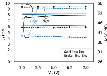
Fig.7 First investigation of bias condition on power gain at high  $V_{cc2}$  and low  $I_b$
