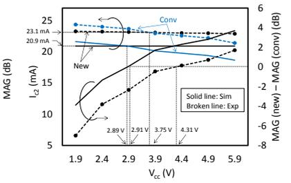
Fig.10 Second investigation of bias condition on power gain difference at low  $V_{cc2}$  and high  $I_b$
