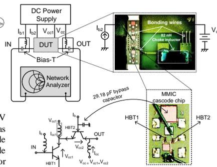
Fig.6 Experimental setup
