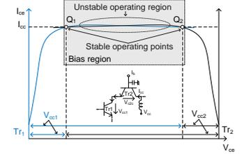
Fig.3 Bias condition of conventional cascode structure with two stable bias points  $Q_1$  and  $Q_2$  where one of two transistors is forced to be biased in saturation region, so the other must be biased in saturation region. In other words, bias point cannot be set independently.
