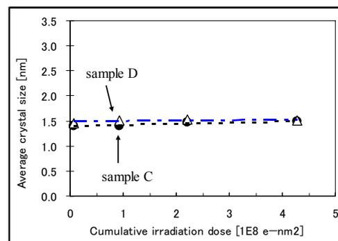
Fig. 2 Effects of electron-beam irradiation on the crystal size of the samples.
