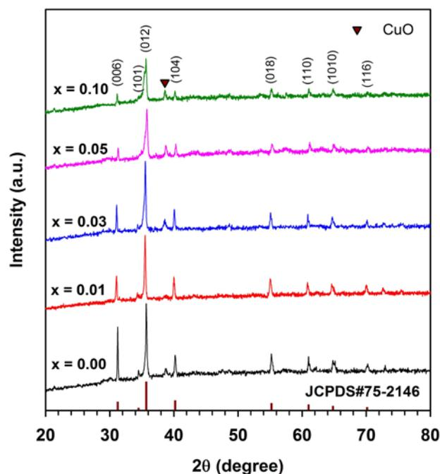
Fig. 1 The XRD patterns of the  $\text{CuFeO}_2$  and the  $\text{CuFe}_{1-x}\text{Ge}_x\text{O}_2$  specimens with Ge content of  $x = 0.01, 0.03, 0.05$  and  $0.10$ .
