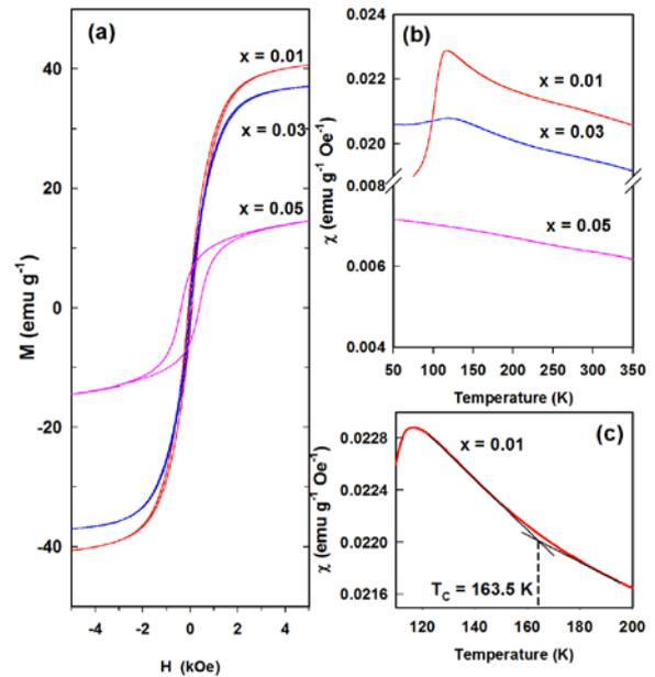
Fig. 3 (a) M-H curves of  $\text{CuFe}_{1-x}\text{Ge}_x\text{O}_2$  samples measured at 50 K. (b) Temperature dependence of ZFC susceptibility of  $\text{CuFe}_{1-x}\text{Ge}_x\text{O}_2$  samples at 0.15 T. (c) The extracted Curie temperature for  $x = 0.01$  sample.
