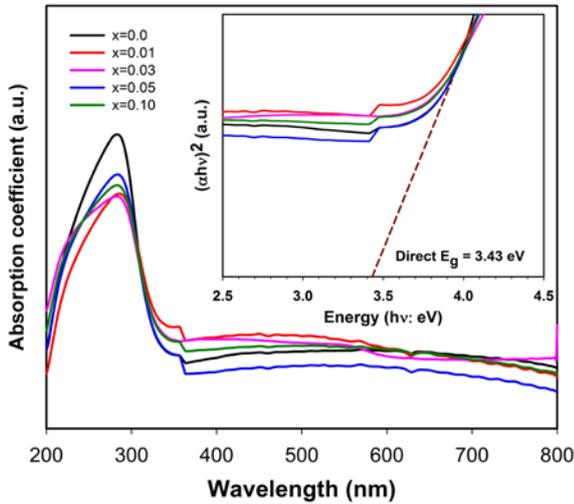
Fig. 2 The absorption spectra of the  $\text{CuFe}_{1-x}\text{Ge}_x\text{O}_2$  samples at room temperature. The direct optical band energy gap is in the inset of figure.
