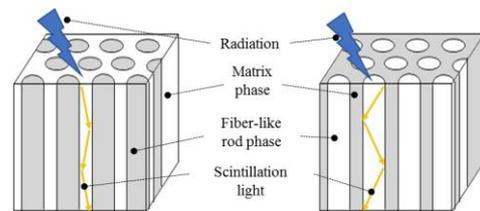
Fig. 1. Schematic view of PSSFs for light-guide system.
