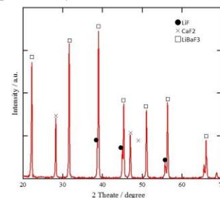
Fig. 3. The powder XRD pattern of the grown eutectic
