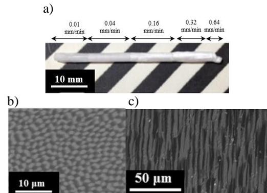
Fig. 2. Structure of LiF/CaF<sub>2</sub>/LiBaF<sub>3</sub> ternary eutectic scintillator, a) photograph of LiF/CaF<sub>2</sub>/LiBaF<sub>3</sub> ternary eutectic scintillator fabricated by micro-pulling down method, b)BEI of transverse cross-section of the polished crystal, c)BEI of vertical cross-section along the growth direction of the polished crystal.
