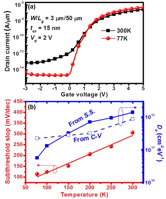
Fig. 3 (a) Transfer characteristics of a MOSFET with an array of Ge-QD/SiO<sub>2</sub>/SiGe-shell heterostructures. (b) shows the temperature-dependent subthreshold slope and corresponding *D<sub>it</sub>*.
