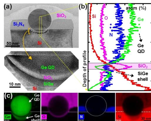
Fig. 1 (a) TEM images as well as EDX elemental (b) line-scanning and (c) mapping examinations of a Ge-QD/SiO<sub>2</sub>/SiGe-shell heterostructure on the Si substrate.
