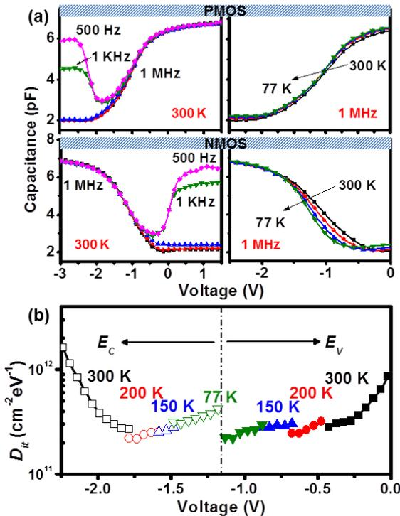
Fig. 2 (a) *C-V* characteristics as a function of frequency and temperature and (b) the extracted *D<sub>it</sub>* of a MOS capacitor with NiGe/SiO<sub>2</sub>/SiGe heterostructures.
