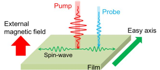
Fig. 1 Schematic illustration of spatially resolved pump-probe technique. Spot diameter of pump and probe beam are  $2.5 \mu\text{m}$  and  $1 \mu\text{m}$ , respectively. Probe beam was scanned to detect spatially dependent spin-wave signal.
