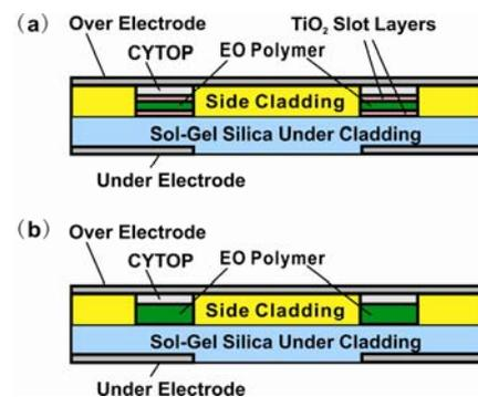
Fig. 1 Schematic cross-sectional view at the active region. (a) The EO polymer/TiO<sub>2</sub> multilayer slot waveguide modulator. (b) The hybrid EO polymer/sol-gel silica waveguiding modulator.
