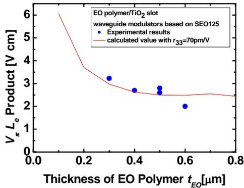
Fig. 3  $V_{\pi}L_e$  product with respect to the thickness of the EO polymer (SEO125). The blue close circles show experimental results and red line shows calculated one by 3D FDTD method.
