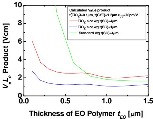
Fig. 2  $V_{\pi}L_e$  product with respect to the thickness of the EO polymer (SEO125) calculated by 3D FDTD method. The thickness of the TiO<sub>2</sub> and CYTOP is 0.1 and 1.2  $\mu$ m, respectively.  $r_{33} = 70$  pm/V. Red and blue lines show for EO polymer/TiO<sub>2</sub> slot waveguide modulator with the thickness of the sol-gel silica undercladding of 4 and 1  $\mu$ m, respectively. Green line shows for standard hybrid EO polymer/sol-gel silica waveguide modulator.
