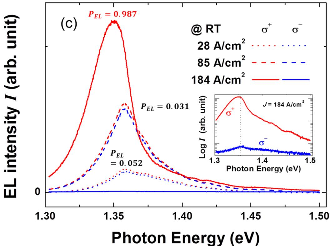
**Fig. 1** : (a) Schematic device structure, (b) experimental configuration, and (c)  $\sigma^+$  and  $\sigma^-$  components of EL spectra emitted from spin-LED at three different current densities,  $J = 28, 85,$  and  $184$  A/cm<sup>2</sup>. The inset shows the same EL spectra at  $J = 184$  A/cm<sup>2</sup> in logarithmic scale to emphasize the spectral shapes.
