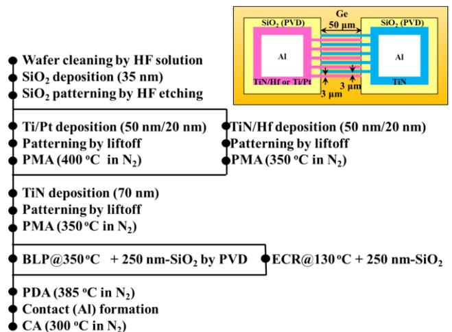
Fig. 1 Fabrication process flow of four asymmetric MGeM diodes.
