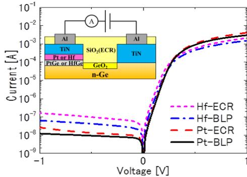
Fig. 2  $I$ - $V$  characteristics for MGeM diodes. Inset shows cross-sectional structure of MGeM diodes and how the  $I$ - $V$  characteristics were measured.
