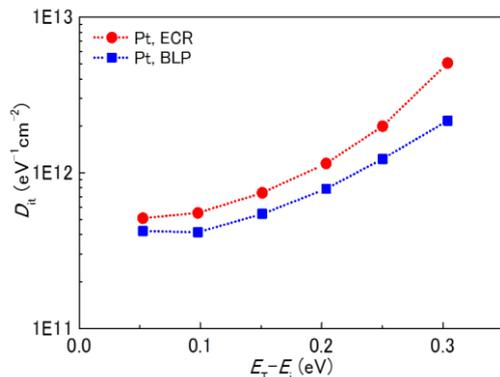
Fig. 3  $D_{it}$  of Pt-BLP and Pt-ECR diodes.  $E_T$  and  $E_i$  are energy positions of interface states and mid-gap, respectively.
