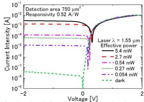
Fig. 5 Dark and photo currents measured under various laser powers using a typical PtGe/Ge/TiN diode with BLP.
